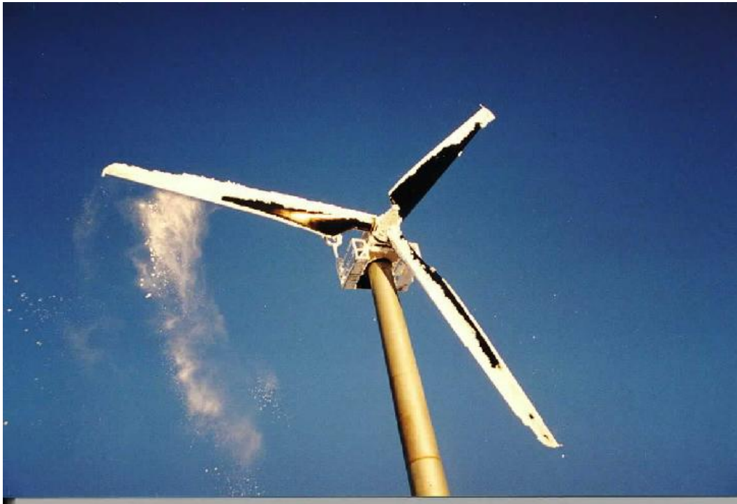
Photograph 8: accumulated ice shedding from black blades
